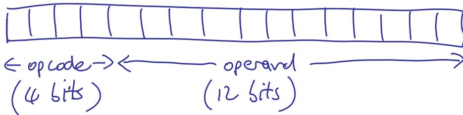
The opcode for ADD is 3 (or 0011 in 4-bit binary) and ADD takes a single operand that is a 12-bit address. So the instruction ADD 27 is:
