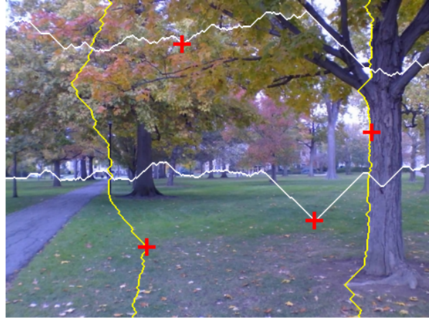
Figure 1. Strongest paths can demarcate perceptually important boundaries, but can also wander through perceptually similar regions or “run away” to distant, strong edges. Two vertical and two horizontal strongest paths are shown, with seed locations as red crosses.
