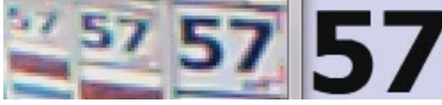
Figure 13: Example of screen capture used to compute display latency. The “57” on the right is displayed directly on the screen, and the reproductions of the “57” to the left are the result of three successive feedback loops through the camera.
