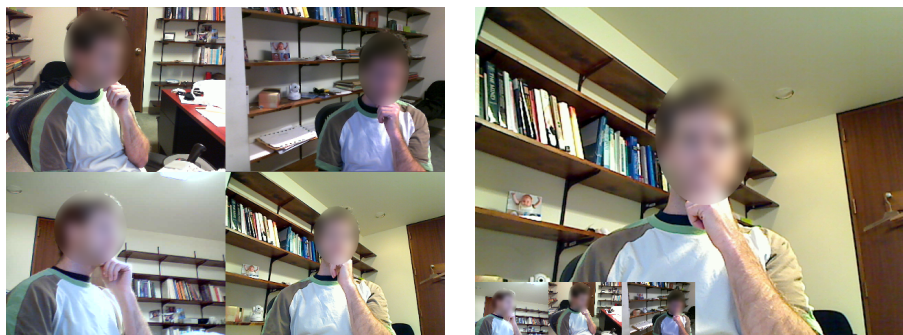
Figure 4: MultiCam's two modes. Left: In the tiled mode, the virtual camera shot contains subsampled versions of frames from each physical camera. Right: In the non-tiled mode, the virtual camera fills the frame with the output from one physical camera, then adds small overlays from the other cameras.
