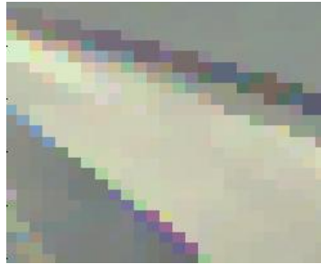
Figure 2.2: The zipper effect is still a serious problem in images demosaiced by the vector median method.
